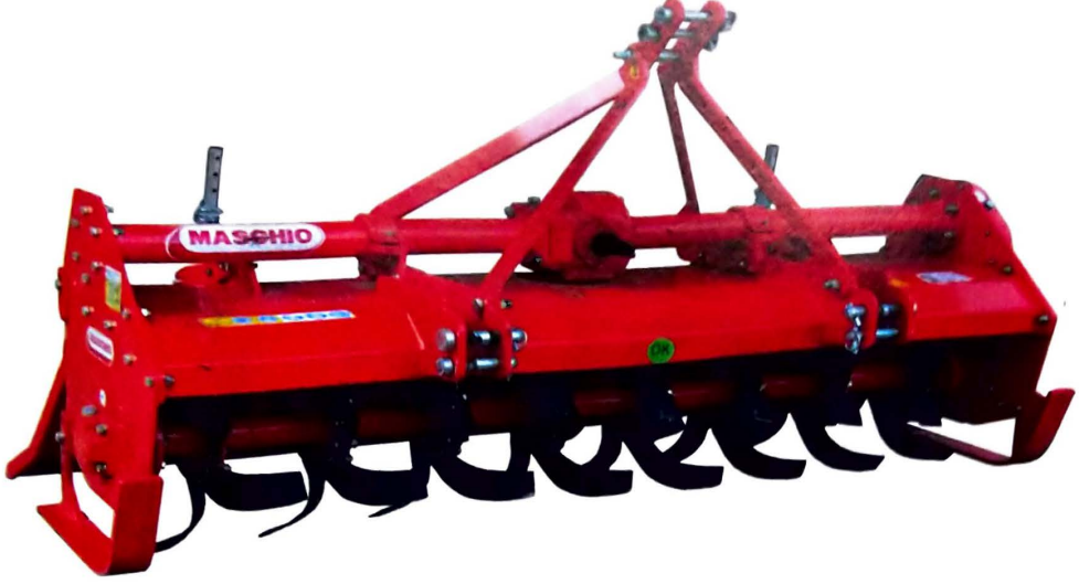
MASCHIO GASPARDO ROTARY TILLER, Model: PADDY 165 (Gear Drive)(Tractor Operated)
