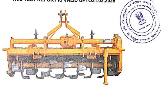
SWAN AGRO ROTARY TILLER (ROTAVATOR), MODEL: NSML RTJT162 MULTI SPEED, GEAR DRIVE, CENTRALLY MOUNTED
