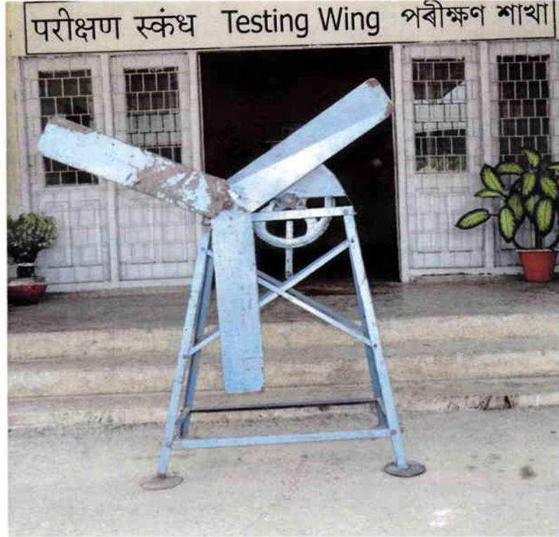
**NBSU WINNOWING FAN, MODEL: WF07 (MANUALLY OPERATED)**
