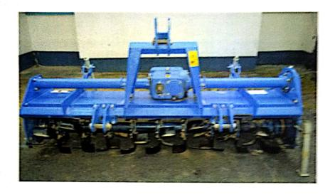
FARMPOWER ROTARY TILLER (ROTAVATOR), MODEL: FPJPMG-185 (ROTAVATOR JYRO+ 6 FEET) MULTI SPEED, GEAR DRIVE, CENTRALLY MOUNTED
