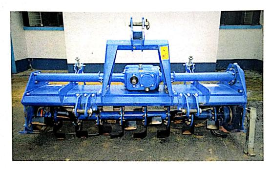
FARMPOWER ROTARY TILLER (ROTAVATOR), MODEL: FPJPMG-160 (ROTAVATOR JYRO+ 5 FEET) MULTI SPEED, GEAR DRIVE, CENTRALLY MOUNTED
