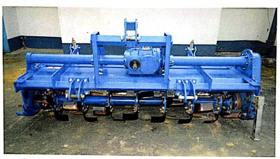
FARMPOWER ROTARY TILLER (ROTAVATOR), MODEL: FPHDMG-185 (ROTAVATOR HEAVY DUTY 6 FEET) MULTI SPEED, GEAR DRIVE, CENTRALLY MOUNTED
