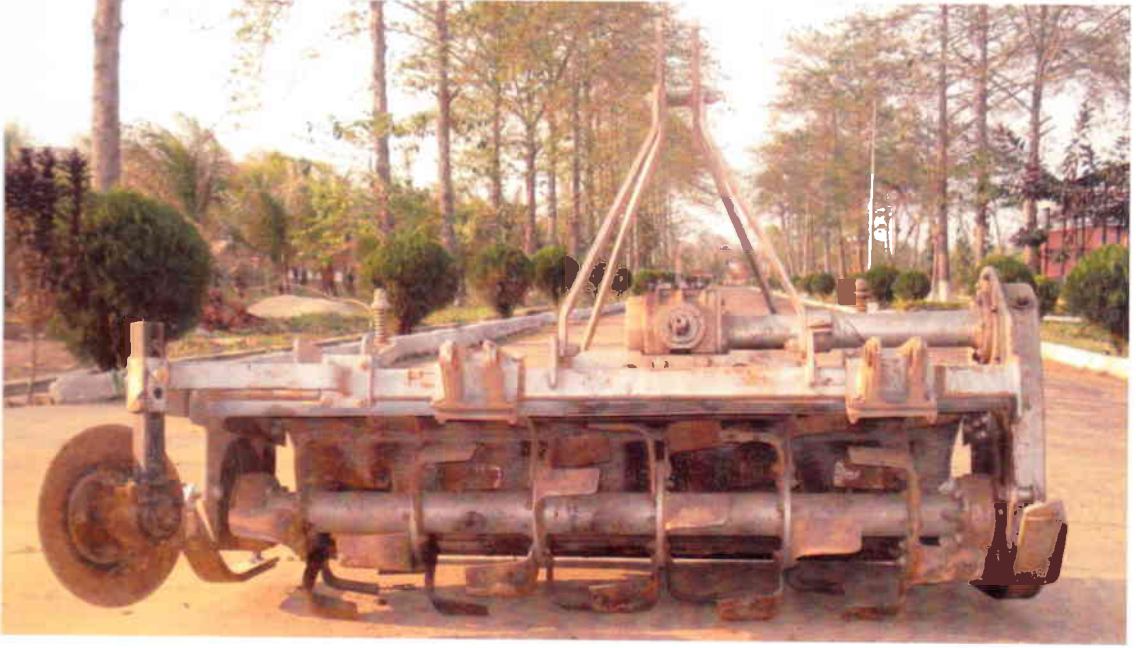
Fieldking FK 150 Rotavator (Tractor-mounted)
